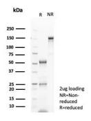
SDS-PAGE Analysis of Purified NeuN Recombinant Mouse Monoclonal Antibody (rNEUN/8054). Confirmation of Purity and Integrity of Antibody.
