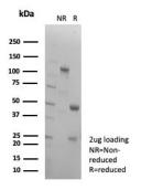
SDS-PAGE Analysis of Purified COL2A Recombinant Rabbit Monoclonal Antibody (COL2A1/8810R). Confirmation of Purity and Integrity of Antibody.
